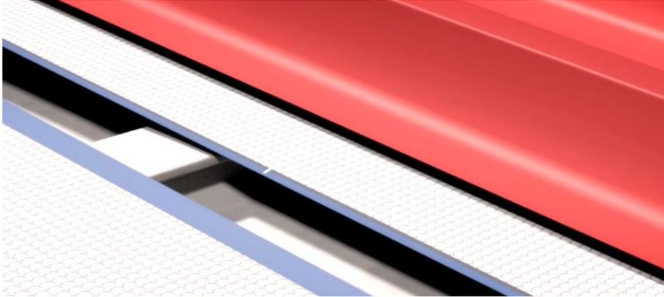
5. Where necessary cut Jumbolene® Roof Insulation around any penetrations making sure to have tight fit to minimize openings.
